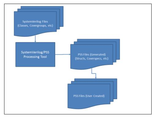
Figure 2 - Typical SystemVerilog to Portable Stimulus Reuse
